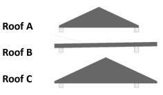
A: Roof with a 25-degree pitch, without overhangB: Flat roof design for a living roofC: Roof with a 25-degree pitch and has a 6 feet overhang.
